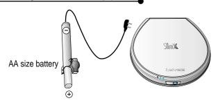
■ The external battery pack can be attached as shown in the figure. Two AA size alkaline batteries are used in the external battery pack.
